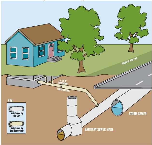
Property owners are also responsible for making sure sump pumps, foundation drains, and roof gutter downspouts are not connected to the sanitary sewer system (see the **Inflow & Infiltration** main page).
